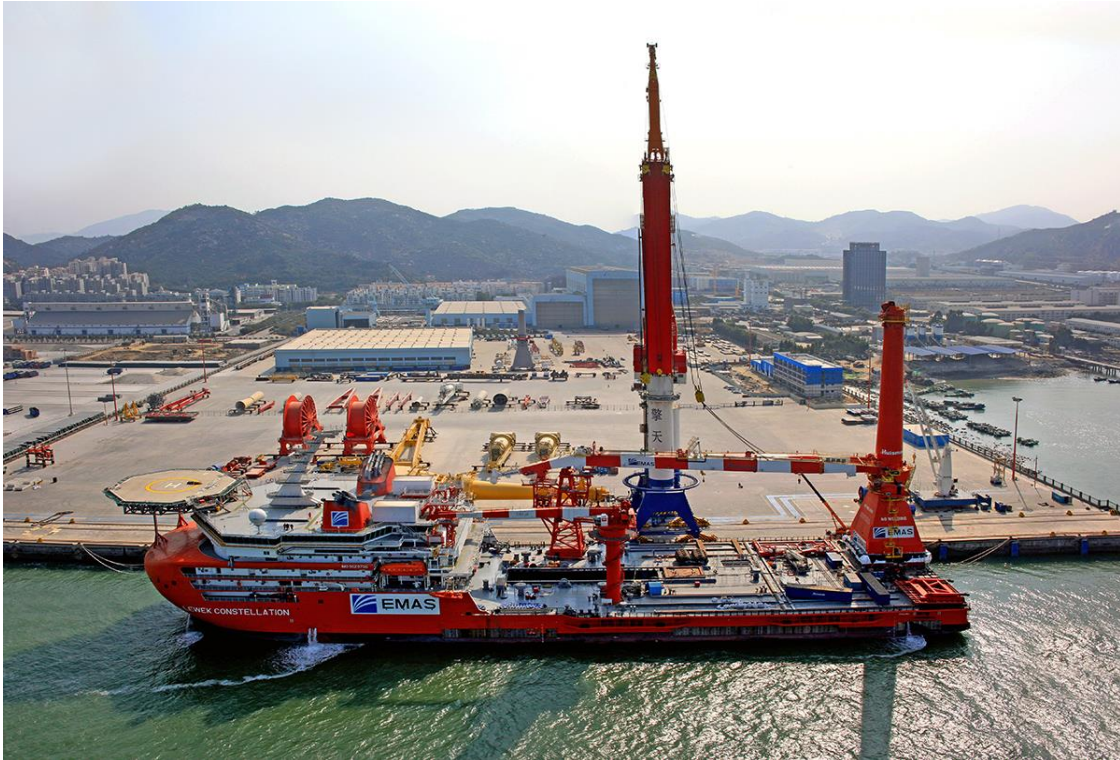
The Lewek Constellation with her 3,000MT crane installed.
