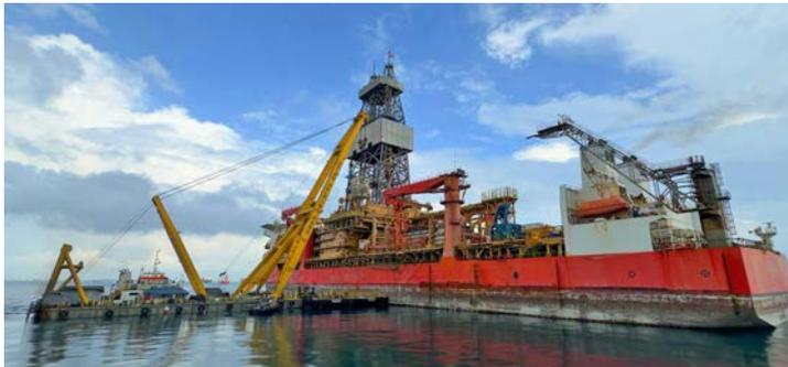
Blowout Preventor & Lower Marine Riser Package offloading in anchorage
