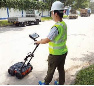
Ground probing radar scanning
