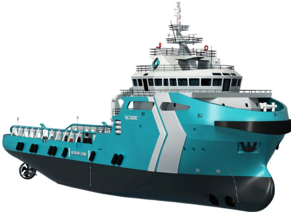
*NCA80E, a 64.8m diesel electric powered AHTS with 80 tonnes bollard pull, based on Nam Cheong's proprietary design*
