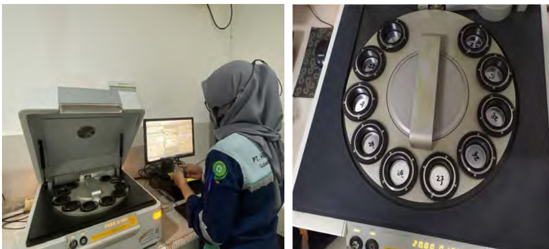
Photo 27 Pressed pellets being loaded into XRF machine
