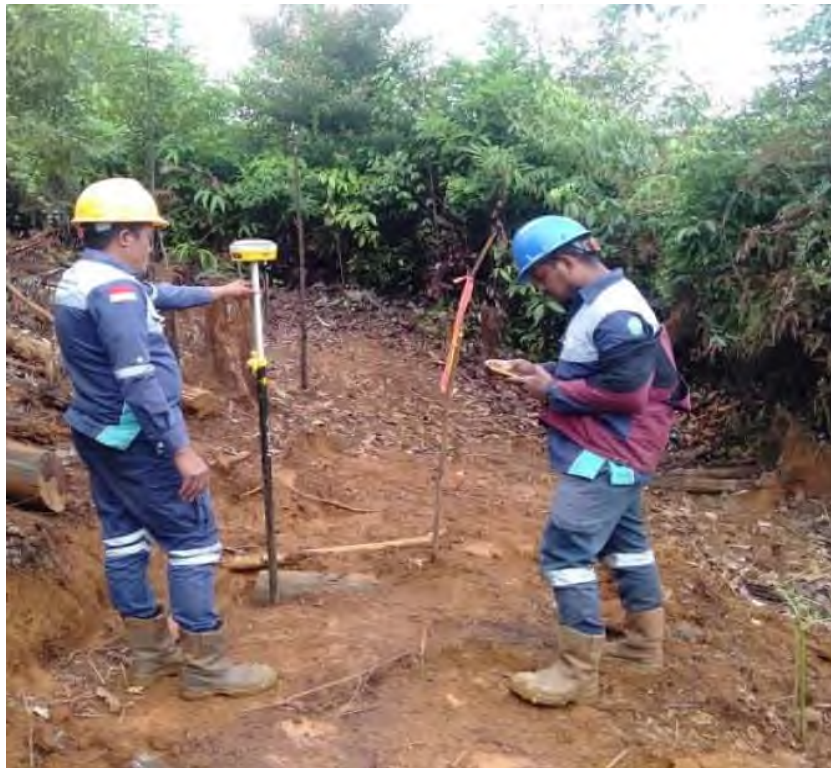
Photo 4 Drill collar survey using E-survey RTK GPS
