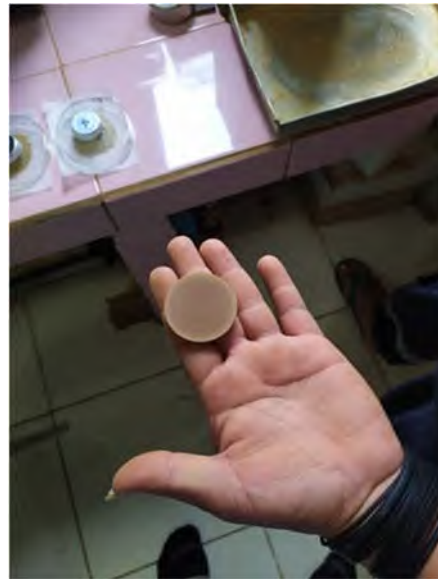
Photo 26 Pressed pellet production from sample pulp ready for XRF analysis
