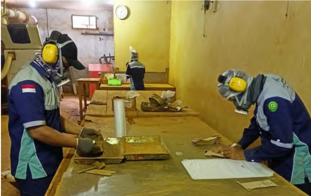
Photo 12 -3mm sample, manual incremental reduction JIS M 8109-1996
