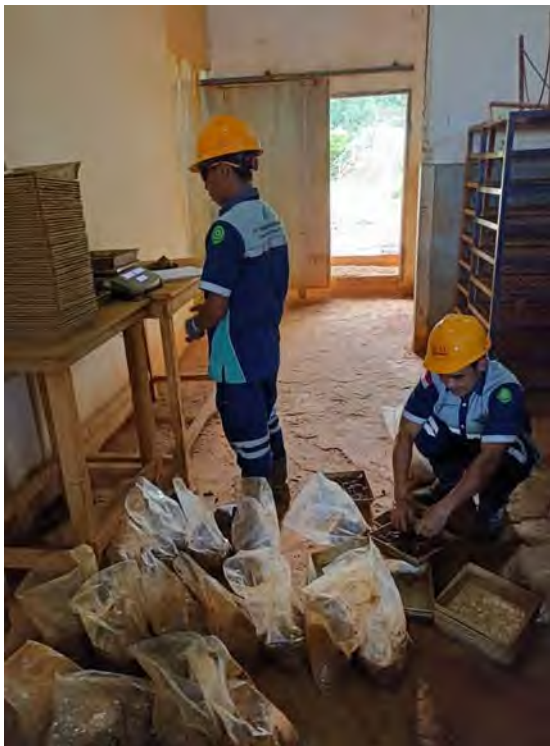
Photo 24 Wet and dry sample weight measurement
