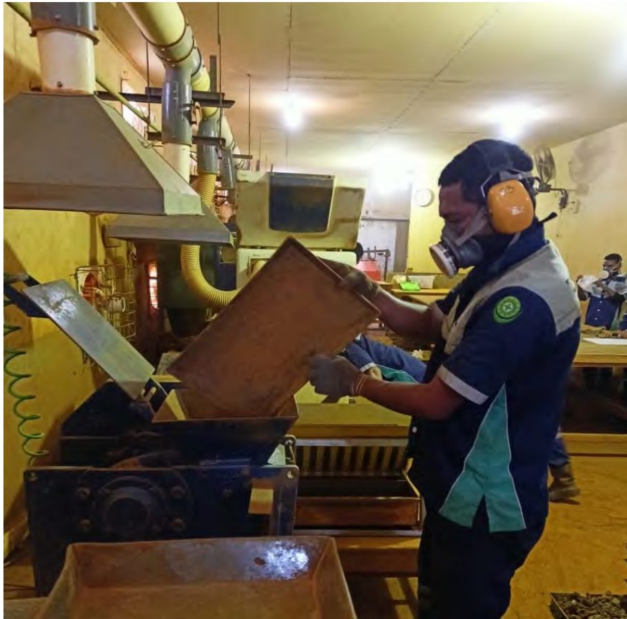
Photo 11 Jaw crushing to -10mm
