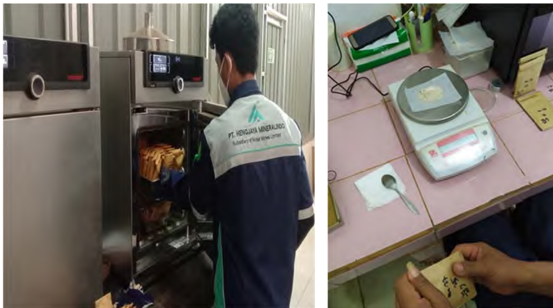
Photo 25 Sample pulp storage in desiccating oven and pressed pellet preparation
