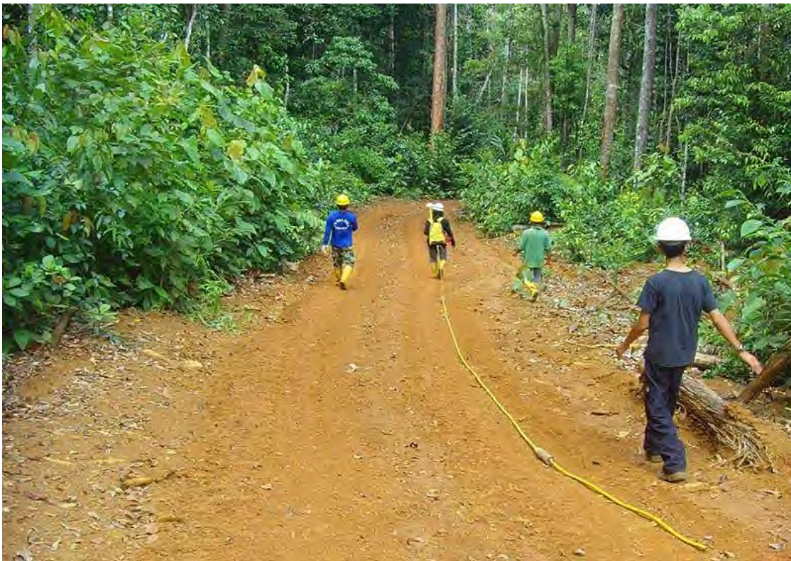
Photo 2 Example survey acquisition using Ultra GPR equipment (source: Groundradar.com)
