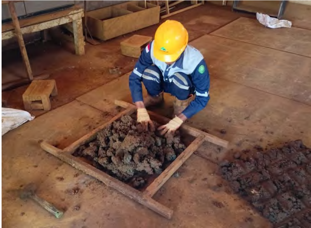
Photo 10 Raw core sample preparation for quartering
