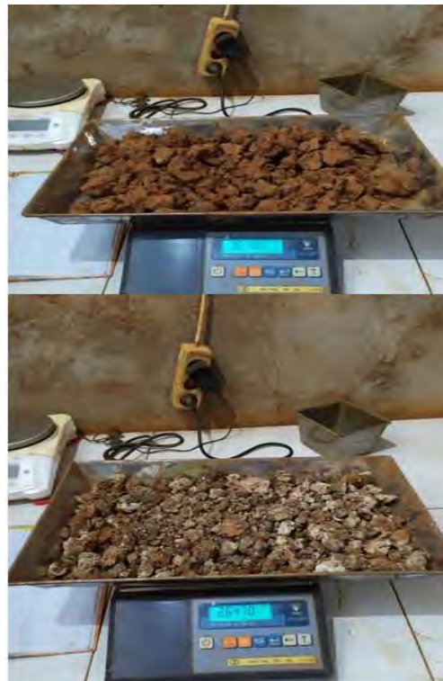
Photo 24 Wet and dry sample weight measurement
