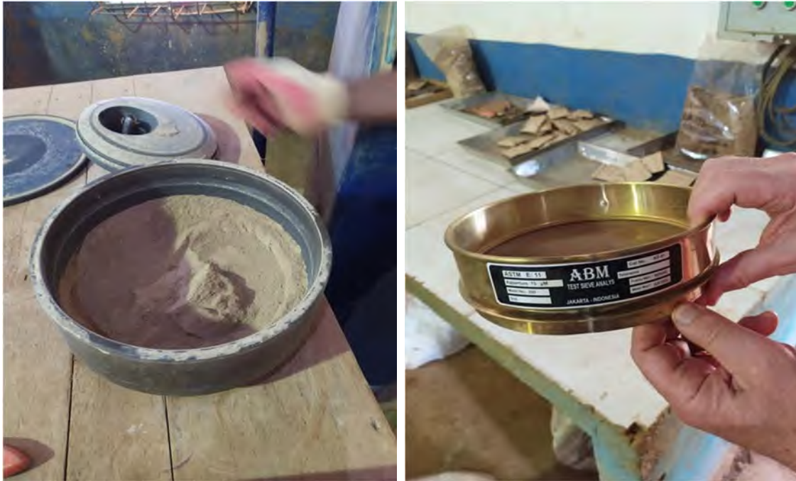
Photo 14 Pulverized sample sieve analysis
