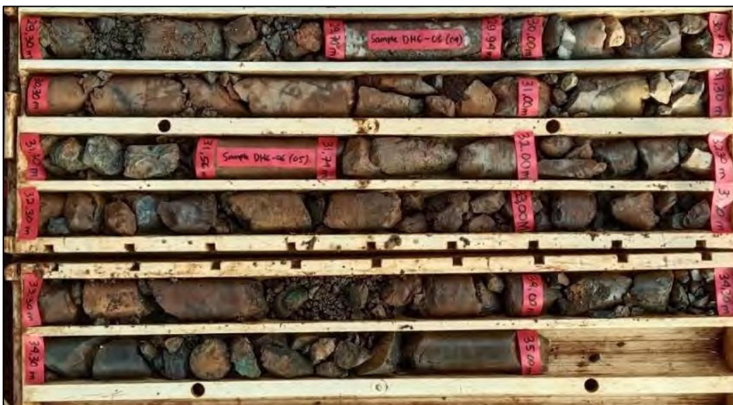
Gambar 4.7 Contoh Material Saprolite
