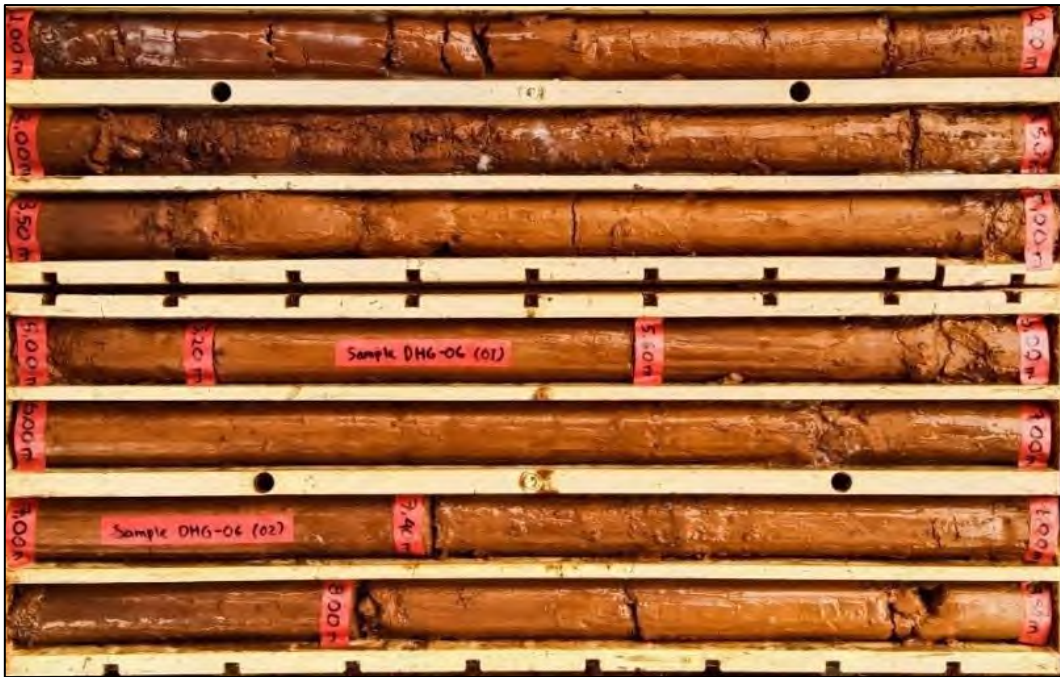
Gambar 4.6 Contoh Material Limonite
