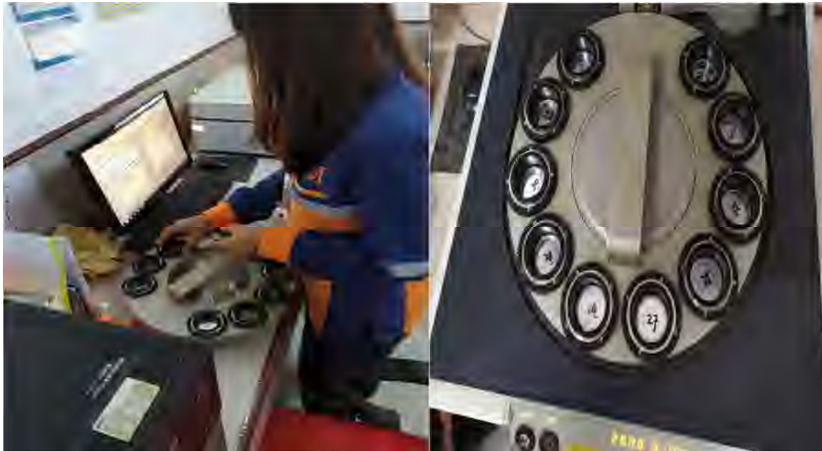
Photo 24 pressed pellets being loaded into XRF machine
