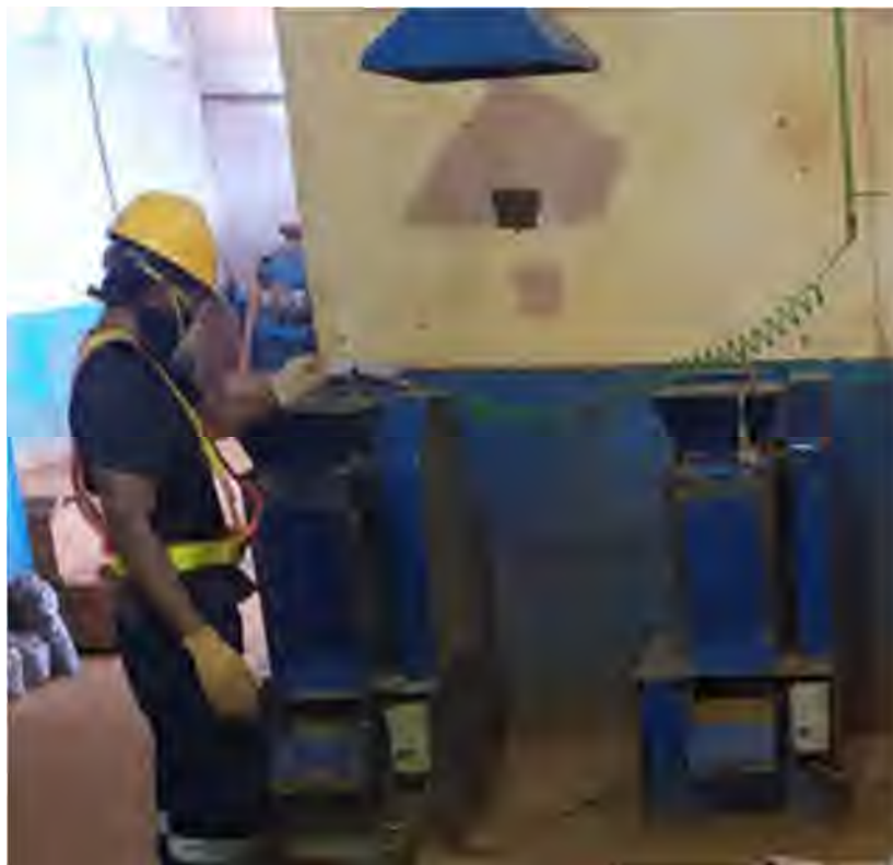
Photo 8 jaw crushing to -10mm
