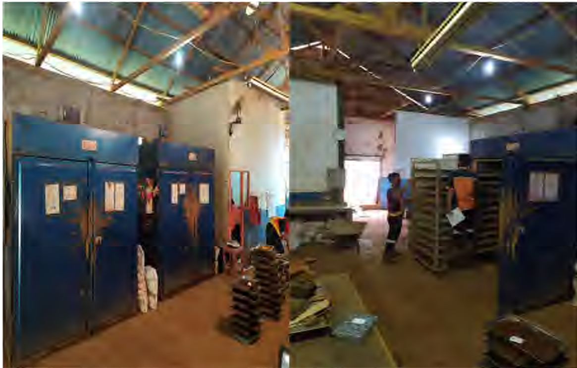
Photo 19 wet samples are placed in oven Photo 20 dry samples removal from oven
