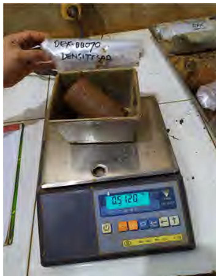
Photo 15 weighing density samples at the sample preparation lab
