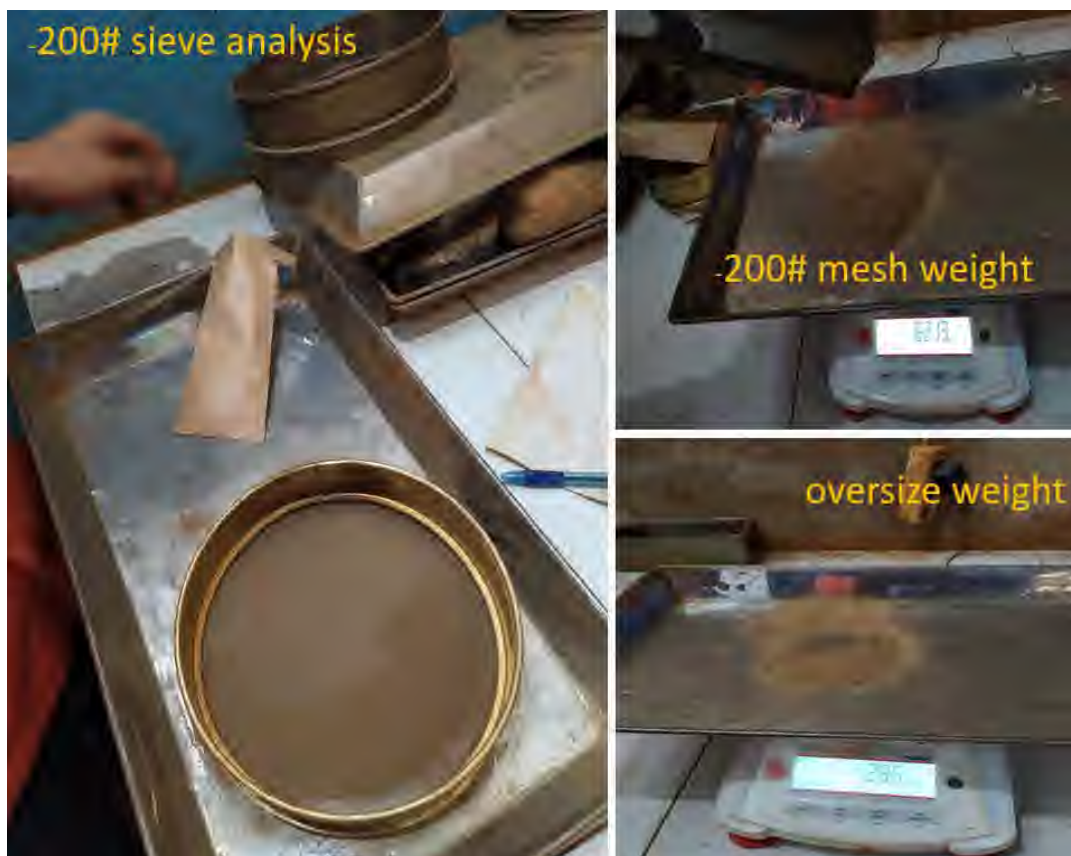
Photo 12 sieve analysis results measurement
