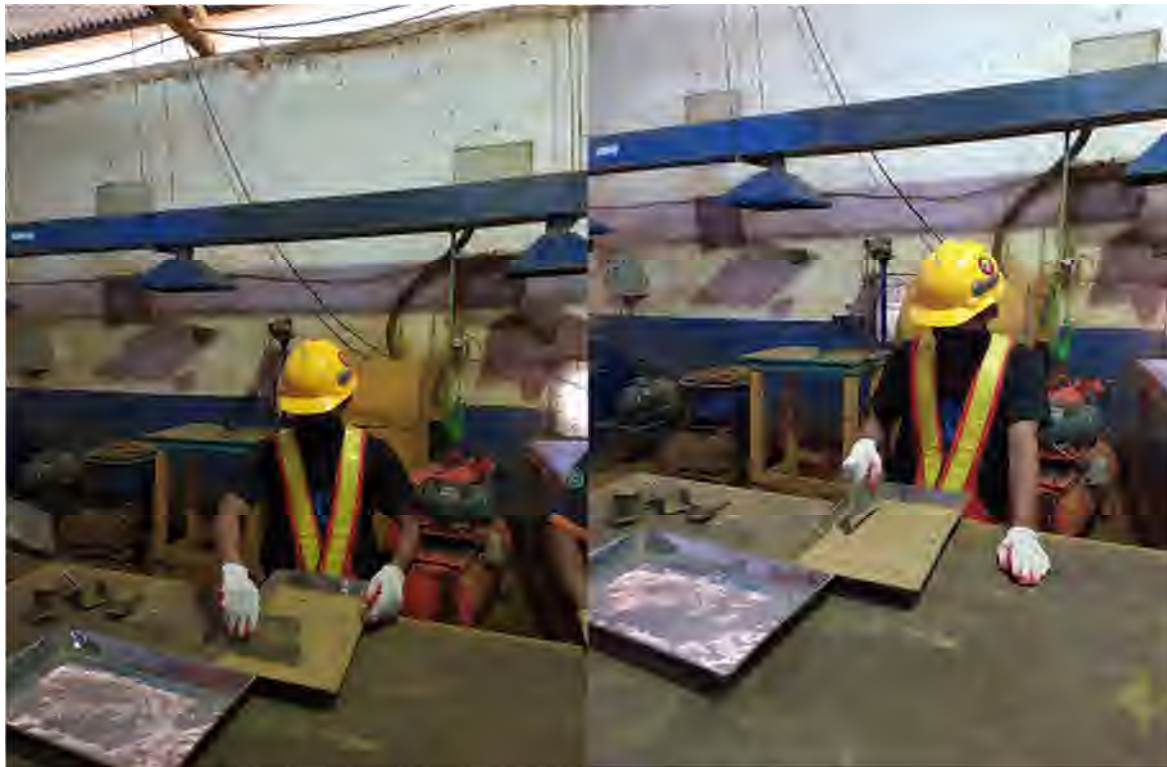
Photo 9 -3mm sample, manual incremental reduction JIS M 8109-1996
