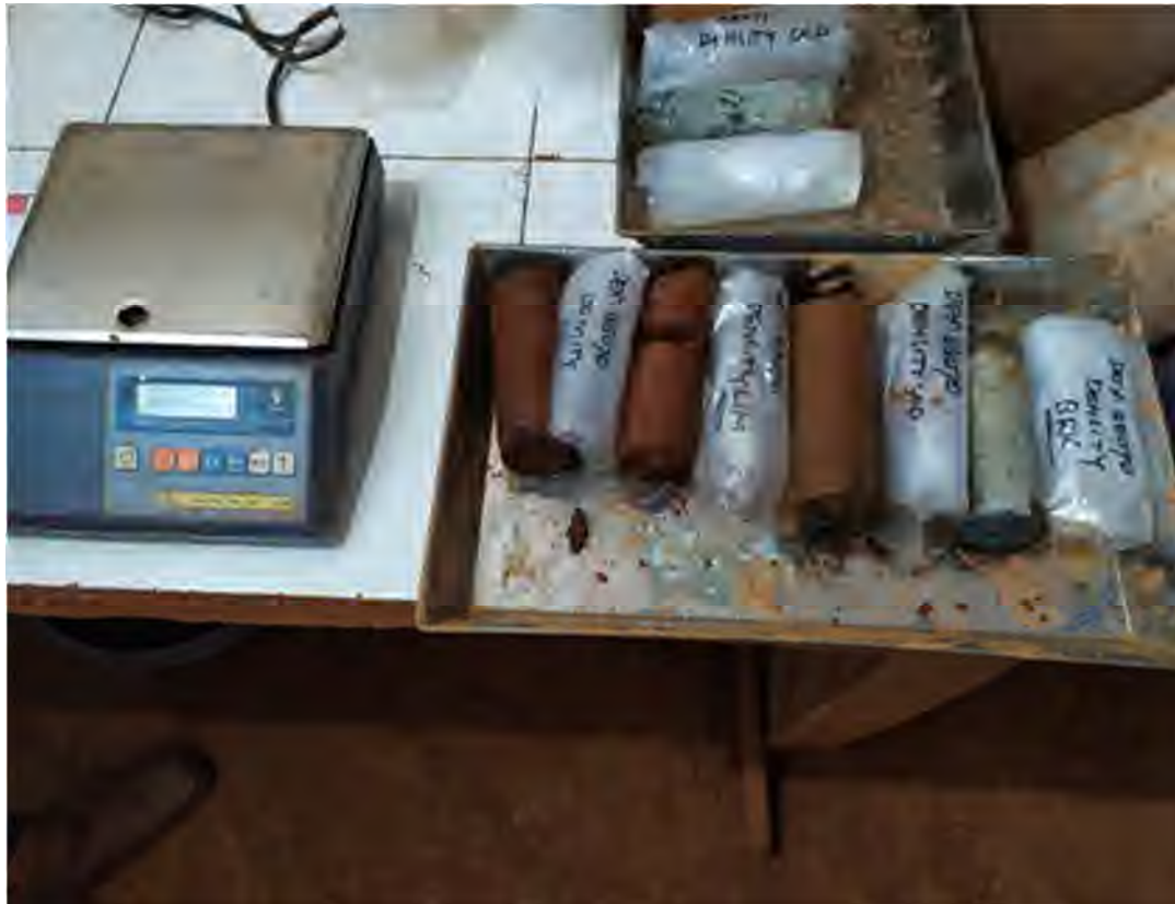
Photo 14 core samples ready for density measurement
