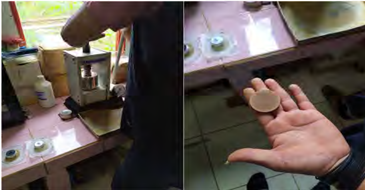
Photo 23 pressed pellet production from sample pulp ready for XRF analysis
