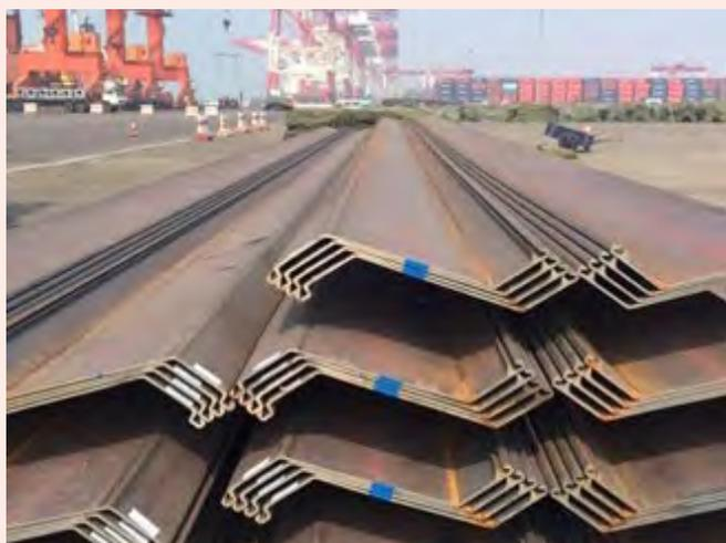
Sheet piles manufactured by MHZ use 20% less steel than traditional sheet piles.
