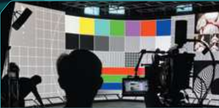
LED screen colour calibration for film production with physical set build, to reproduce a scene atop a helipad
