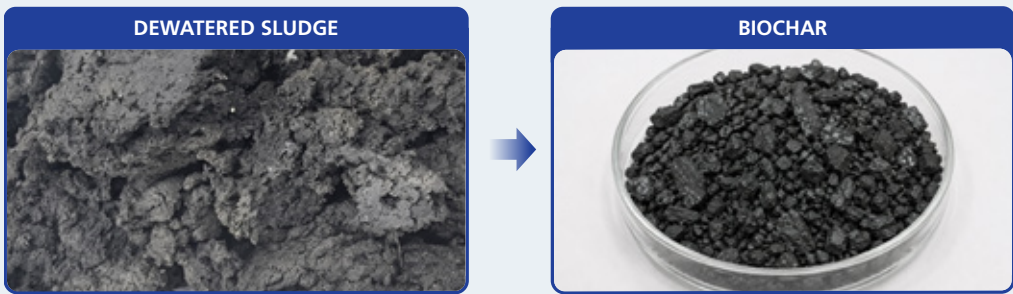
Sludge is converted to biochar through pyrolysis.
