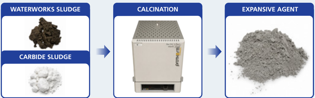
Sludge is converted into an expansive agent through calcination.
