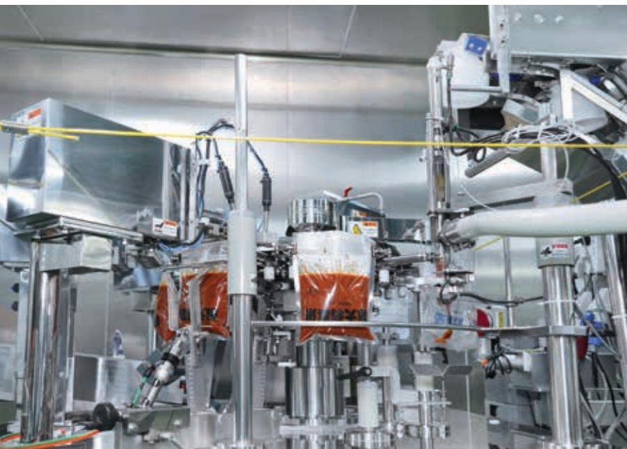
Automated hot-fill conveyor line in Tianjin kitchen
