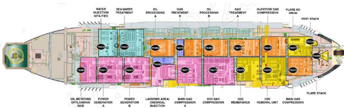
Figure 5-2 – Ihabela FPSO Topsides General Arrangement (1)
