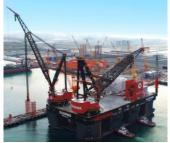
World's largest, strongest and most sustainable semi-submersible crane vessel with a lifting capacity of 20,000 tonnes and dual-fuel powered for Heerema
