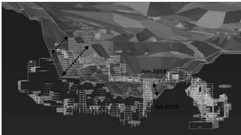
Figure 8-11. Oblique view of resource model showing topographic surfaces at June 2014 and Jul 2019.
