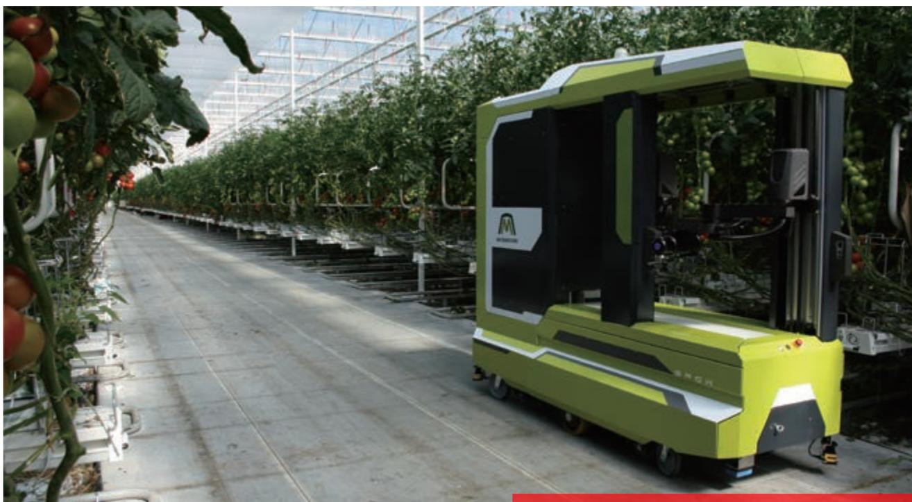
MetoMotion's autonomous greenhouse tomato-picking robot in action.
