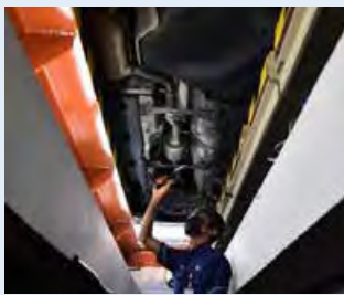
Inspecting undercarriage for oil leaks and ball joints condition.
