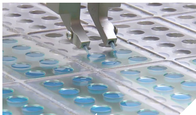
▲ An automated robotic arm dispenses a drug product in liquid suspension form into blister pack wells.
