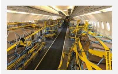
Removed passenger seats from four aircraft (2x SIA 777-300ERs, 2x Scoot A320s) to create **modified freighters**
